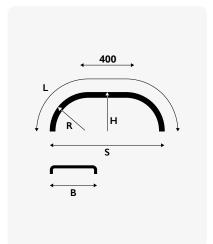
Parlok White Line™ steering axle F400 mudguards are designed for the wheel's extra manoeuvring space and a large span requirement. They are made of three parts ie. 2 x round + 1 x straight piece by welding them together and securing the joints with rivets on the side. The length of the straight part is 400 mm. The range covers all usual lengths and widths for the wheel sizes on steering axle. Available also with integrated spray-suppression.
