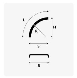
The original Parlok OFF-RD™ mudguard. Made of PE-HD (high-density polyethylene) with a large range of usage temperature and excellent chemical resistance. Strong against wear & tear and light in weight. A wide range of lengths, widths, radiuses and taylor-made solutions can be manufactured to various requirements.
