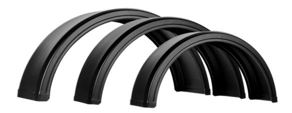
These three sizes with widths 240, 270 and 320 mm are suitable for small single wheels in commercial vehicles.
