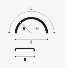
The OFF-RD™ mudguards are available also in a long 160° version, specifically designed for agricultural trailors. Like all Parlok mudguards, also this type is made of PE-HD (high-density polyethylene). We offer a wide range of lengths, widths and radiuses, and can produce custommade solutions to meet various requirements.
