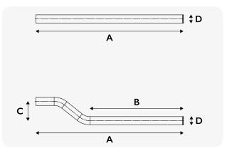
Powder-coated or Zn tube stays with diameter 42 mm, without flange, are suitable for various mounting conditions.
