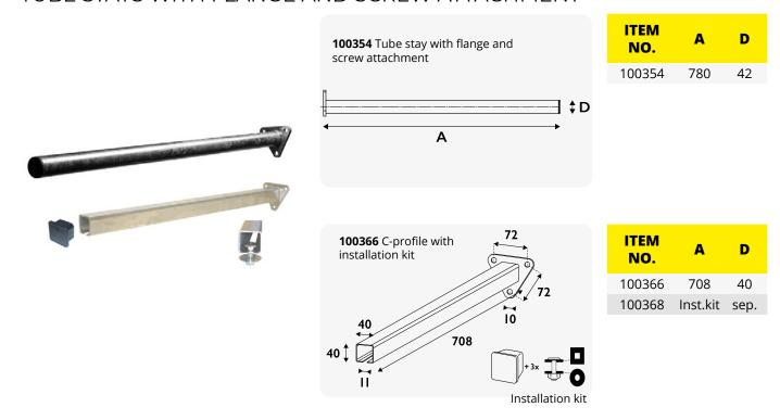
The C-Profile bracket set (100366) is our own innovation popular already for a long time through its' low cost. C-profile is made of zinc-coated steel and is available as a 3-bolt mounting variation. It is especially suitable for narrow installation conditions. The set is delivered inclusive the end plug and installation kit. The installation kit is available also separately with item number 100368.
