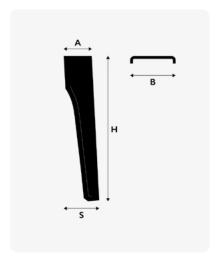
The straight SPAT is very easy to fasten with just screws through the top to a vehicle's plywood bottom plate, for example. No additional support is required. The compatibility especially in the sizes 450x640 mm and 450x730 mm to commonly used spat & valance systems in semi-trailers is a great advantage in the after sales business. The products can also be equipped with Supra spray-suppression.
