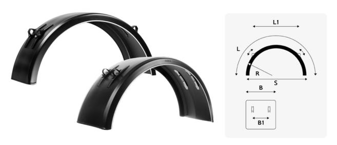
Original Parlok White Line™ with adjustable brackets. The range of adjustment 86 mm for P42 and 65 mm for S42 as well as the option to customise the bracket position offer an unlimited range to fit the mudguard on vehicle. A very strong combination for your mudguard solution with extremely easy installation. Just lift on tube stays and tighten the four nuts.
