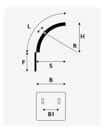
The assembly of the 1/4 mudguard is very easy with the brackets S42 and P42 that secure the quarter mudguard tightly on the tube stay preventing it from spinning. The range of adjustment is 86 mm for P42 and 65 mm for S42.
