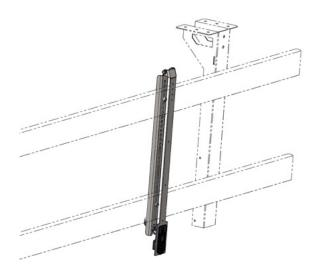
The brackets are designed for easy fitting of Aero panels and deflectors on a vehicle providing the strength of the lateral protection device. A smart locking mechanism allows an easy opening or lifting off of the panels when access to the underside of the chassis is needed. The lightweight but strong-built brackets feature a smart-looking and reliable locking mechanism. Attachment can be adjusted according to the bar distance.
