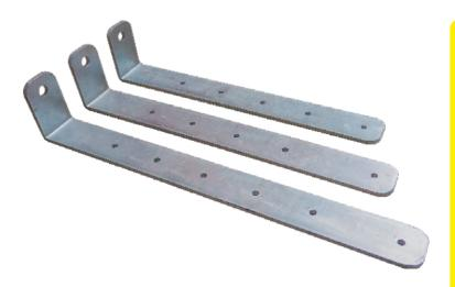
The flat brackets are made of 8 mm Strenx® 650 MC hot-rolled high-strength structural steel (HSS), and the surface treatment is hot-dip galvanising (70 µm).
