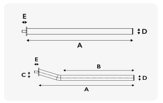
We can provide you a wide range of powder-coated tube stays with diameter 42 mm for various mounting conditions. Tube stays are made of steel and they are black polyester powder-coated. Pretreatment is made with ecological zirconium process. The tube stays are available with an M16, some even with an M14 screw.
