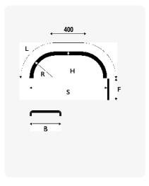
Parlok White Line™ steering axle mudguards for the wheel's extra manoeuvring space, with integrated spray-suppression. The length of the straight part is 400 mm.
